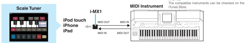
By using a Yamaha i-MX1, connect the instrument to an iPod touch, iPhone, iPad.
