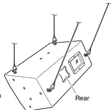
**EN** Incorrect examples for suspended installation
