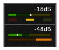
Dynamics 1 is displayed at the top of the thumbnail with Dynamics 2 at the bottom. (Output channels have only Dynamics 1.)
