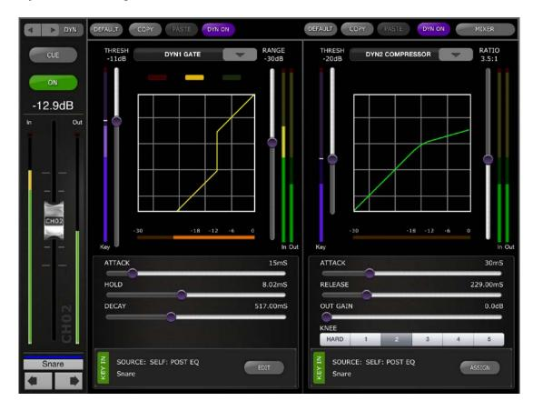
The left side of this screen (Channel Strip) is identical to the EQ Editing screen with channel fader, On button, Cue button, input and output meters, channel name, color and navigation buttons.
