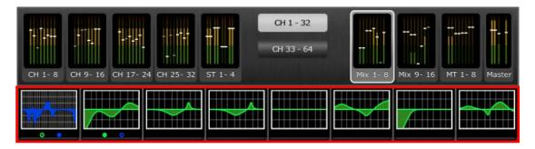
Green and blue dots below each EQ curve indicate the types of EQ available on that channel, and the type of EQ (PEQ or GEQ) that is currently displayed for that channel. A green dot indicates PEQ and a blue dot indicates GEQ. When only PEQ is currently available on a channel, no dots will appear below the curve. (In Demo mode, GEQs appear on Mix busses1, 7 and 8).
