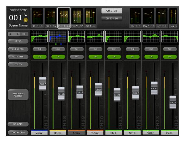
Across the top of the screen, level meters and faders are displayed in blocks of channels for mono Input Channels 1-32, Stereo Input Channels 1-4, Mix and Matrix busses, and the Master Stereo and Mono busses. This is the "Navigation/Meter Bridge".
