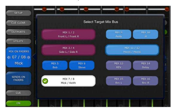
Select the Target from Mix 1-16. The currently selected Mix will appear as a white button with a check mark. Stereo pairs appear as single large buttons.
