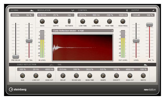
The early reflections are responsible for the spatial impression in the first milliseconds of the reverb. For emulating different rooms, you can choose between different early reflections patterns and adjust their size. The reverb tail, or late reverberation, offers parameters for controlling the room size and the reverb time. You can adjust the reverb time individually in 3 frequency bands.
