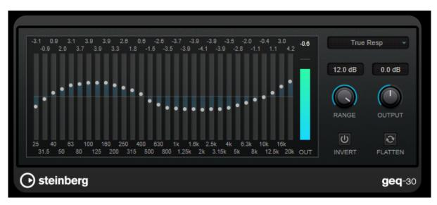
Each band can be attenuated or boosted by up to 12 dB, allowing for fine control of the frequency response. In addition, there are several preset modes available that can add color to the sound of GEQ-30.
