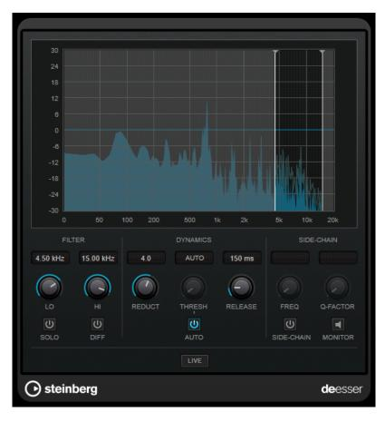
You can use it, for example, when close proximity microphone placement and equalizing lead to situations where the overall sound is just right, but where unwanted sibilants occur. When recording a voice, the position of DeEsser in the signal chain is usually after the microphone preamp and before a compressor/limiter. This keeps the compressor/limiter from unnecessarily limiting the overall signal dynamics.
