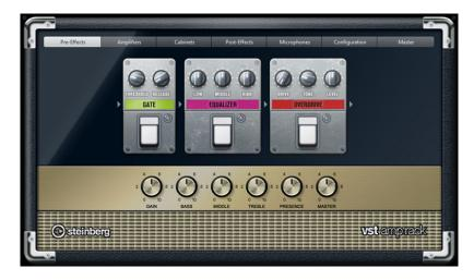
At the top of the plug-in panel, there are seven buttons, arranged according to the position of the corresponding elements in the signal chain. Each button opens a different page in the display section of the plug-in panel ([Pre-Effects], [Amplifiers], [Cabinets], [Post-Effects], [Microphone], [Configuration], and [Master]).
