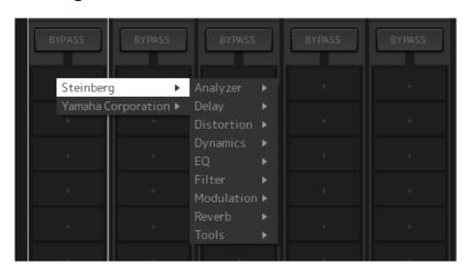
Left-click on an empty slot to display the list of plug-ins. Drag the mouse through the list, and click the desired plug-in name to assign that plug-in to the slot.
