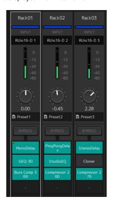
You can drag racks to reorder them within a bank. When doing so, channel assignments do not change. Each bank can contain a maximum of 16 racks, whether Mono or Stereo. If the maximum number is exceeded when you bring in a rack from a different bank, the last rack in the bank (the rack in the rightmost position) moves to the next bank. The same applies if the maximum number of 16 racks is exceeded when you unpair two
