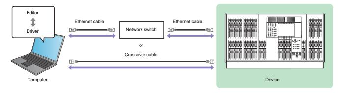
**NOTE** When you connect the computer to the M7CL directly, use a crossover cable.
